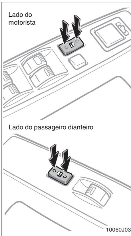
**TRAVANDO E DESTRAVANDO COM O INTERRUPTOR DE TRAVA ELÉTRICA DA PORTA TRASEIRA**
