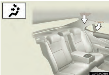
Cool air flows from roof vents.
